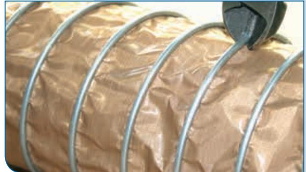
Pull both ends of the hose apart and cut the reinforcement helix using wire cutters.
