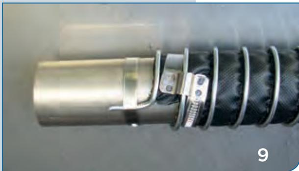
Now attach the appropriate clamp and pull tight so that the metal clip profile is pressed firmly onto the pipe and the hose is fixed in place. There must be contact between the metal clip profile and the pipe.
