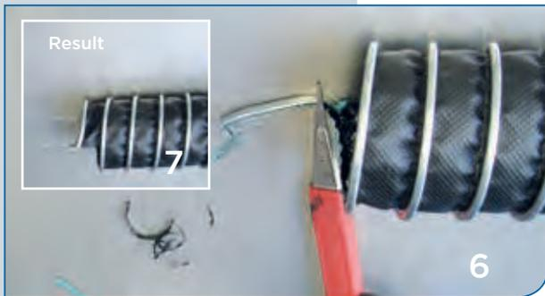
Remove any remaining material from the metal clip profile.
