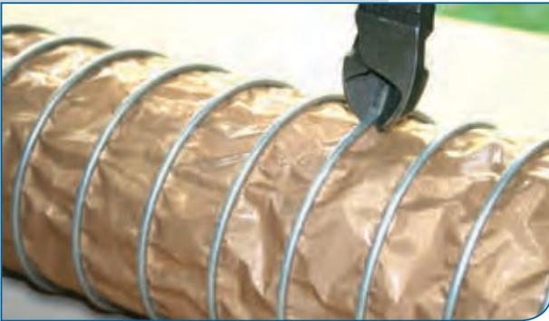
Using a sharp knife, cut the hose material through to both adjacent helices.
