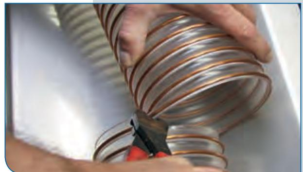
Finally, cut off the hose material cleanly along the reinforcement spiral.
