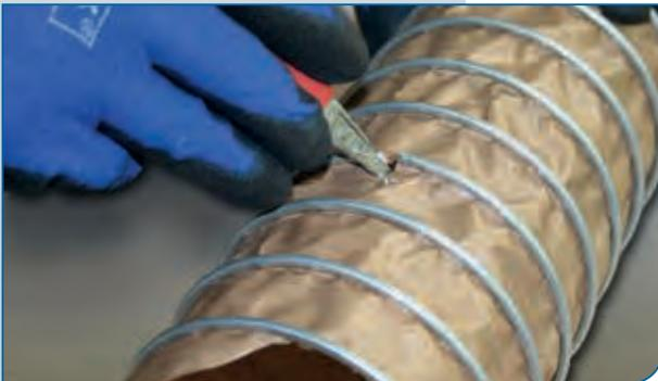
Finally, cut the hose material cleanly along the clip helix.
